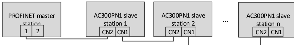
Figure 3.1 Schematic diagram of string connection
